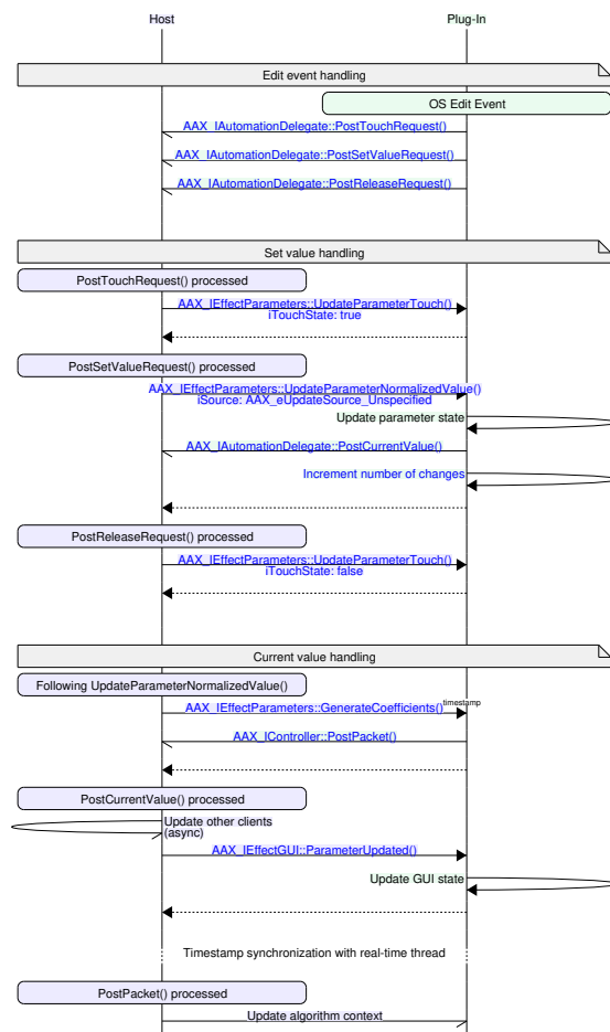
Figure 12.8: High-level sequence of interface calls and events for a parameter update following a user-generated edit
